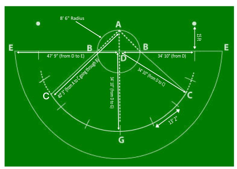
Start at D. Put in a nail and dash out the circle. Make clear dashes at both B's and the A. Move the nail to A.
